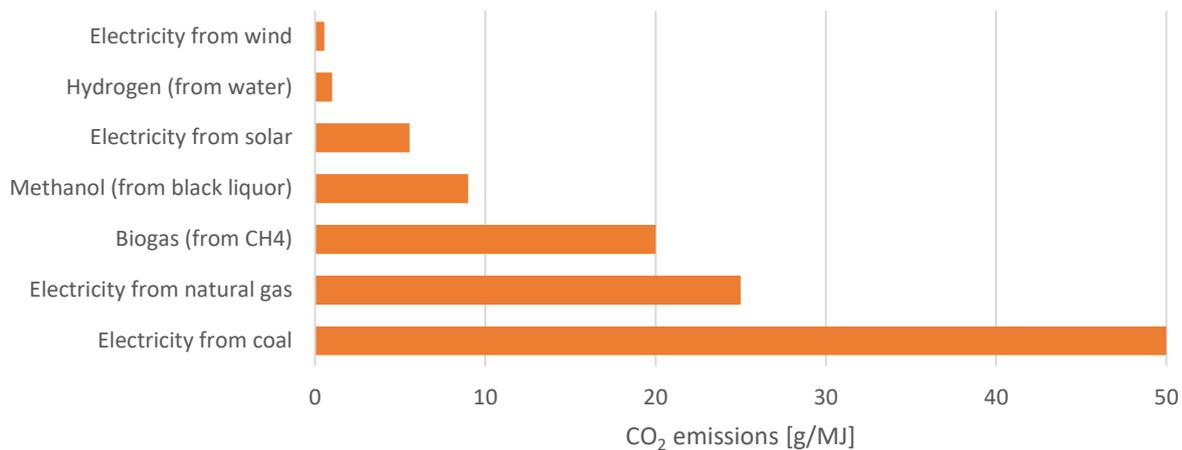
Figure 2 Electricity from renewable sources offers more WTT CO<sub>2</sub> reductions than the least emitting alternative fuels. Data source: (10) and (12)
