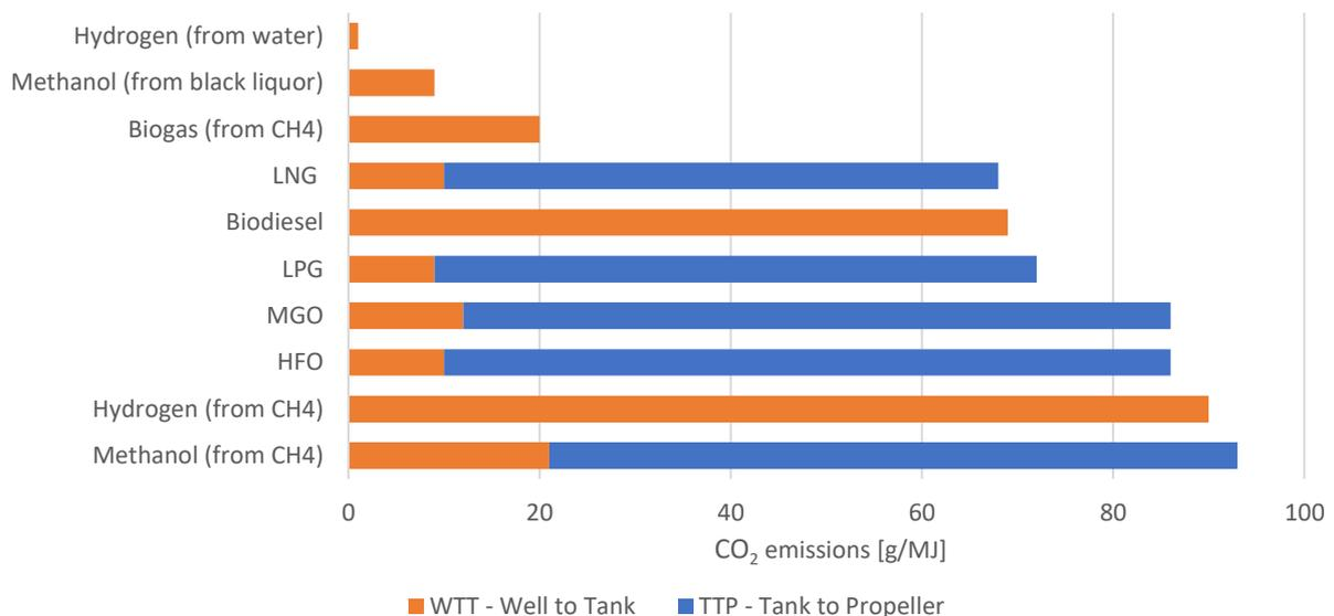
Figure 1: Renewable hydrogen, methanol and biogas offer the most CO<sub>2</sub> reductions of all alternative fuels considered. Graph adapted from (10)
